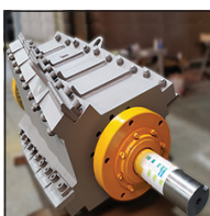
Rotor with 4 angled rows of replaceable striker bars
