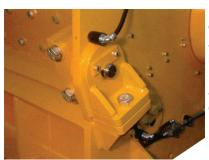
Grate, anvil, and upper frame are **electronically interlocked** to ensure maintenance personnel safety as well as remote monitoring during operation.
