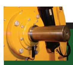
Extra heavy duty swing away anvil with bolt-on liner for ease of replacement.
