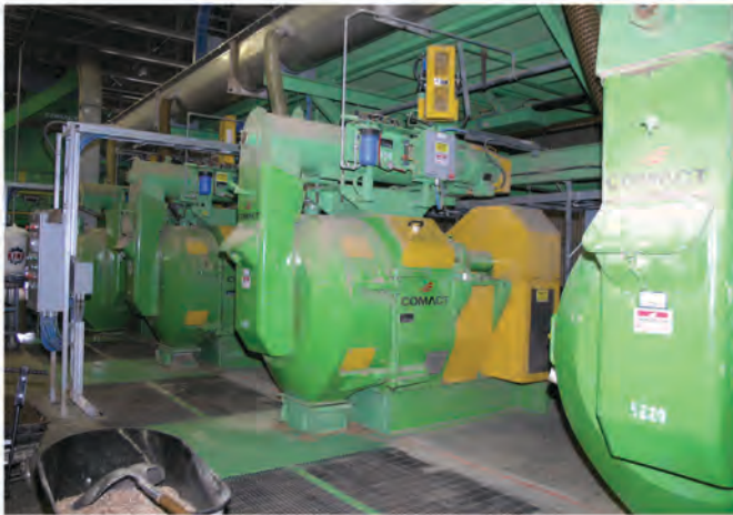
Pelletizing is via five Promill pellet mills supplied by Comact. The mills are designed for fast maintenance access and to avoid lubricant contamination of the final product.
